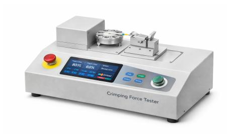
JRAGRAU Crimping Force Tester is designed for accurate measurement of crimping force in wire harness, terminal, and connector applications. The system ensures repeatable, reliable results using a servo-driven loading mechanism and real-time digital monitoring.
